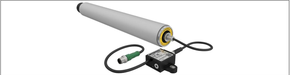
Mainly on inclined conveyor lines, it is important that drives such as the RollerDrive EC5000 hold material to be conveyed in position during stationary conveying operation. If the system voltage fails, the drives are no longer able to do this.
