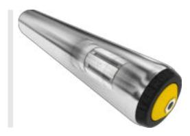
The magnetic speed controller MSC 50 is a purely mechanical speed controller that ensures a controlled, slow speed on gravity conveyors with materials weighing from 0.5 kg (1 lbs) to a maximum of 35 kg (77 lbs). The magnetic speed controller operates without a gear box, thus enabling startup for very lightweight containers. Heavy containers are transported at a controlled speed thanks to the consistently high braking performance.
