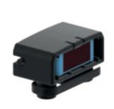
Sensors detect materials on the conveyors and determine their position. Reflex light barriers are used, which require a reflecting mirror (reflector) on the opposite side of the light barrier in order to return the light beam.
