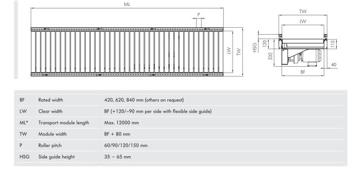
\*If a slave curve is driven by a straight conveyor, the max. module length is reduced by 3000 mm, for 2 curves by 6000 mm.
