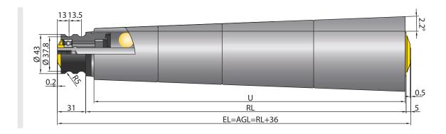
Tapered elements with 1.8° and 1/2" polymer double sprocket head with 14 teeth
